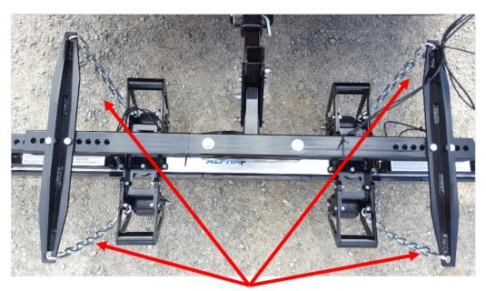
Connect the 4x hanging chains with 8x quick links provided as shown above. The chains must go from the outside of each outrigger to the inside of the appropriate hanging point above it.
