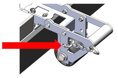
Connect the lower end of the chain in the hole location on the outside of each outrigger as shown above.
