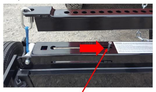
When you have reached the upward position you are satisfied with, slide the contact limit block inwards towards the center of the sweeper (all the way over until you hear the limit block contact the limit switch) and tighten the bolt with a 7/16" wrench. Repeat for opposite side. You have now set the upward travel limit.
