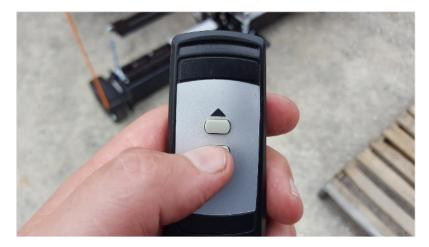
Install Batteries in the remote (2x AAA). Press the down button to extend the blue ropes out as far as possible.
