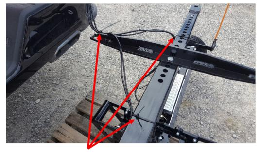
Tie and Secure wires as needed with the provided Cable Ties. Leave enough slack in the wire for travel up and down.
