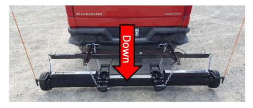
Press the down button on the remote until the chains are tight.
