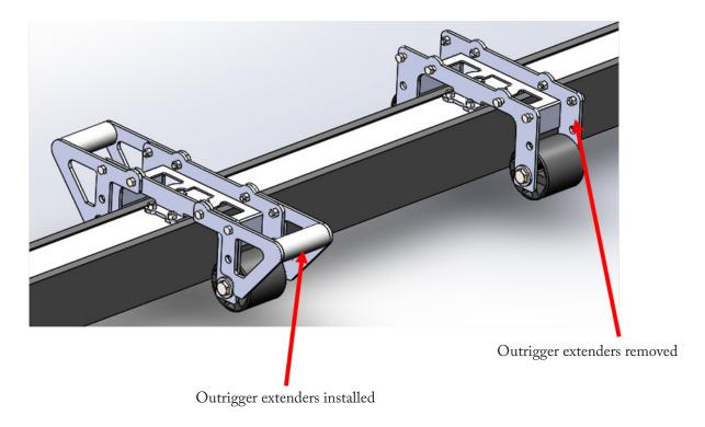
If you chose to install the outrigger extenders, Install Each extender using the provided 3/8" x 1" hex bolts (4pcs) and 3/8" nyloc nuts (4pcs).
