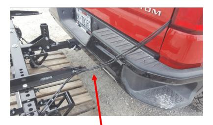
Route the Wires and Connect to a 12v Battery source on your vehicle.
