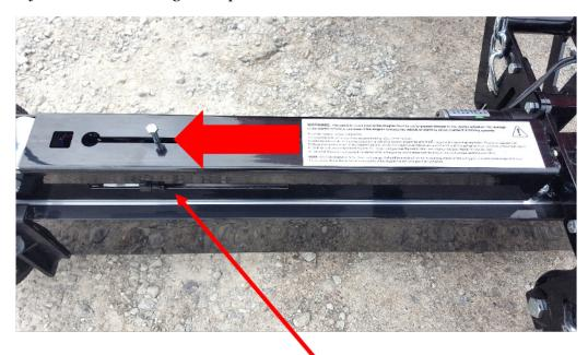
Slide the limit contact block outwards until it contacts the other contact block. Repeat for opposite side.
