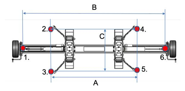
Optimal Dimensions between Suspension Mounting Points
