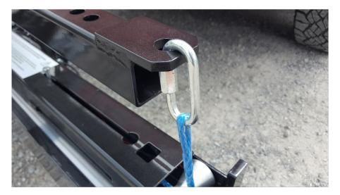
Connect the quick link on the end of each blue rope to the lifting location above it. Pressing the down button on the remote will extend the rope so you can clip it in place. Tighten the nut on the quick link firmly.
